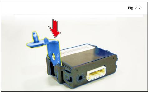
b. Attach the GBS ECU Bracket to the GBS ECU.
